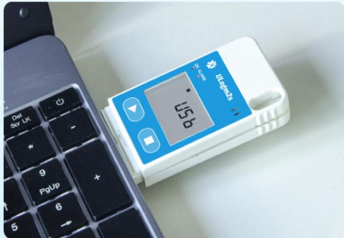
1. Press and hold until the screen displays SET under stop recording mode.
